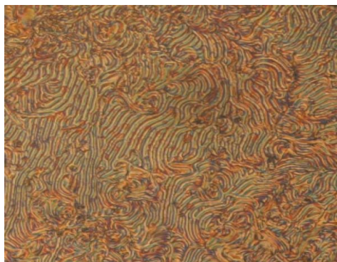
Plate 2. Worm like texture observed in 9BAO+12BAO.
